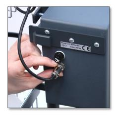
Secure the plug by tighten the thred
