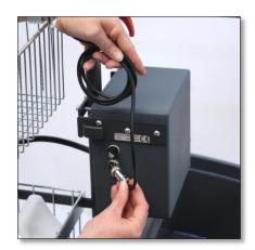
Take the cable from the computercontrol and plug into the grey box in the connector
