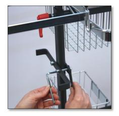
Mount the attachment for the large grey box about 20 cm below the red locking handle.
