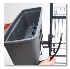
Place the spraybox in the spraybox holder and make sure that the hose is free
