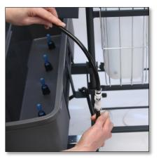
Put the hose ends from the grey box and the spray box togheter with the quick couplings
